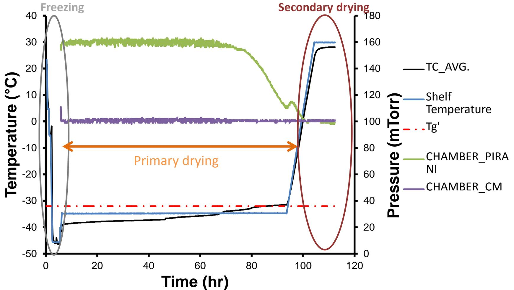
The three phases of a typical lyophilization cycle: Freezing, primary drying and secondary drying
