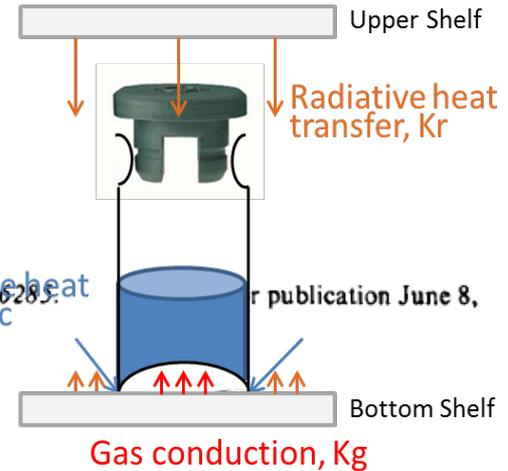
1. Heat and mass flow during freeze-drying is influenced by the vial [heat transfer coefficient ( $K_v$ ), stopper resistance]
