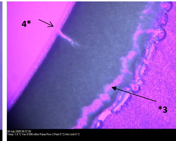
Collapse - temperature too high
