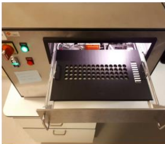
Fig. 1 View of NIR hyperspectral camera. The open drawer shows the plate with 50 positions on which the samples need to be placed for analysis.
