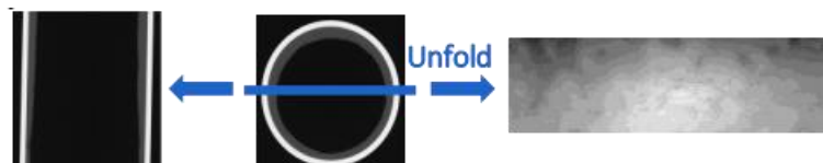
Fig. 2 Unfolded image of the frozen product layer during primary drying
