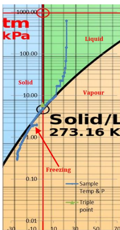
Fig. 1 Showing the Temperature and Pressure profile of a sample of water evacuated in the drying chamber without any cooling of the shelves super imposed upon the phase diagram of water.
